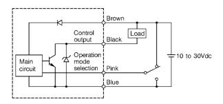
• (PNP output type) polarized retroreflective model, thru scan model receiver, diffuse scan type
